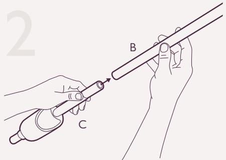
Insert the pole (parts A & B) into the bayonet area on the rear of the mop reservoir (part C) until it clicks
