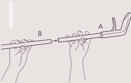
Line up the handle pole (part A) with the additional pole (part B) and push the notch into the insert until it clicks
